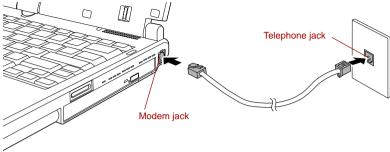
Figure 4-29 Connecting the internal modem
